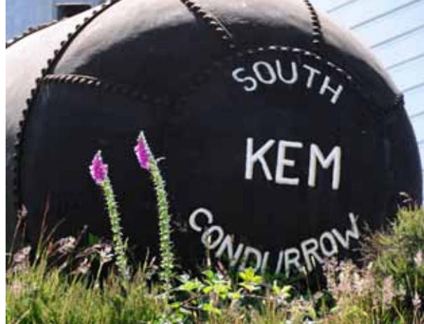
Above: Egg-ended boiler at King Edward Mine
